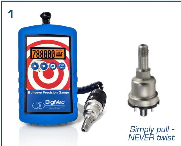
Remove the sensor tube from its cable, making sure that you pull (NOT twist). Then, position the sensor upside down with its threads facing up.
