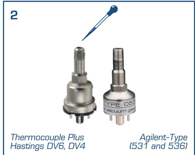
Funnel about a tablespoon of solvent\* into the stem of the sensor. Hold your finger over the vacuum interface and shake the solvent inside the sensor tube.
