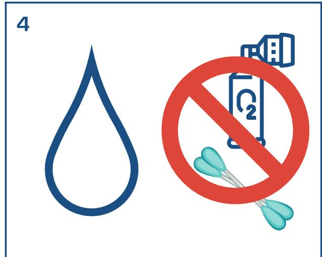
When clean of contaminants, the solvent should run clear out of the sensor tube. Let the sensor air dry. Do NOT dry the sensor after cleaning with compressed air or a cotton swab.
