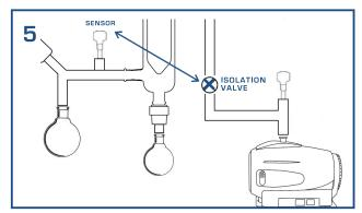
The valve will open and close based on the pressures that Sensor B reads
