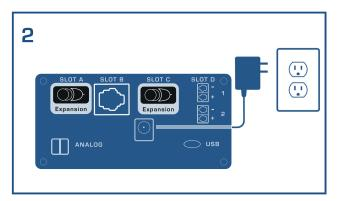
Plug StrataVac into wall outlet using the power supply supplied by DigiVac
