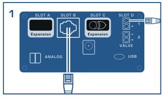
Connect sensor cable to Slot B and connect the valve to Slot D (top)
