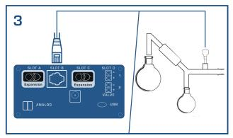
Take sensor and mount it as close to the reaction as possible
