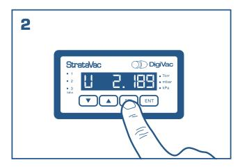
Use the up/down arrows to change the set point. Once the desired set point is reached, press Enter (ENT) to save.
