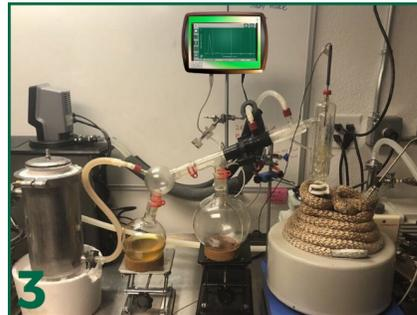
Connect and power the system, then prepare distillation as you typically would
