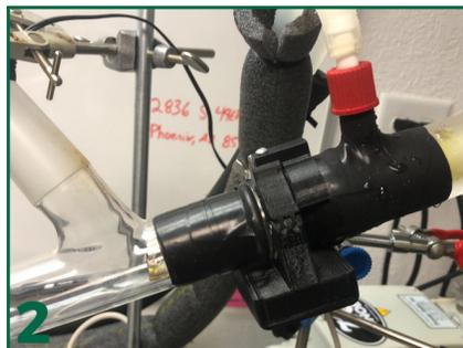
Install the optical sensor with the thicker part of the sensor down
