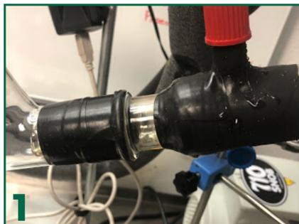
Apply the light blocking tape to your condenser, leaving a gap for the sensor
